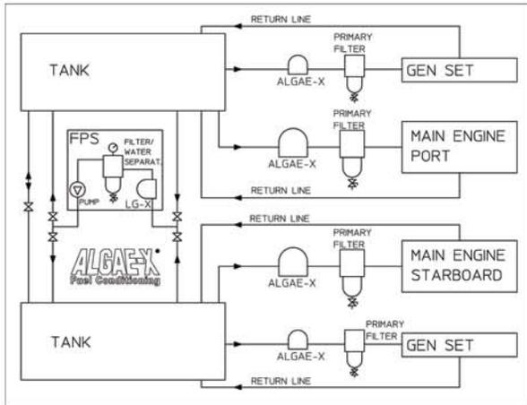
Free and emulsified water will accelerate fuel break down and is detrimental to modern diesels. Water may enter the fuel system during re-fuelling through leaks or as a result of condensation.
