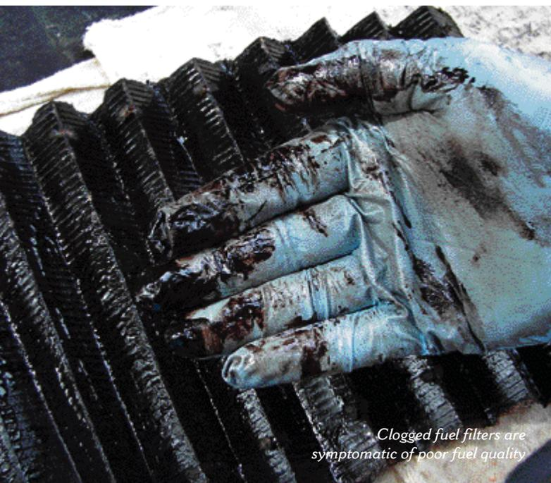
*Clogged fuel filters are symptomatic of poor fuel quality*
