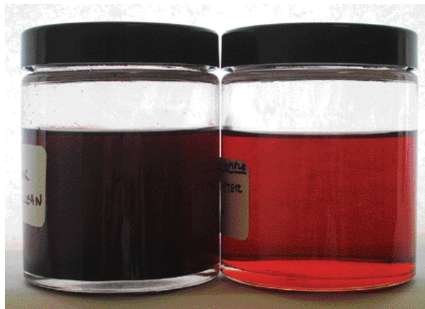
Above left: fuel before and after treatment with an Algae-X fuel polishing system; Above right: fuel production has changed since 1972; Below left: fuel molecules, although tiny, cluster together to form larger particles; Below right: sludge accumulated in a fuel tank
