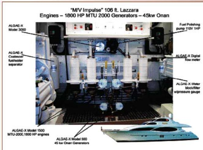
*An Algae-X Total Fuel Management System in situ; it conditions fuel by removing water and debris, improving fuel stability and preventing the build up of the solid organic compounds that cause blockages*
